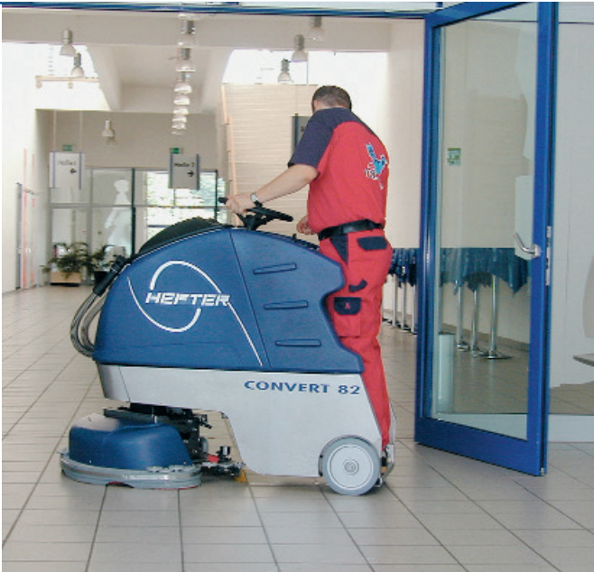
Distinguishing feature: The operator rides in a standing position on the cleaning system. This is not only convenient; it also provides a very clear view on all sides.
